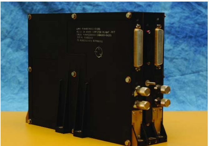
Standard RAD6000 onboard computer, dual or triple processors and power supplies
